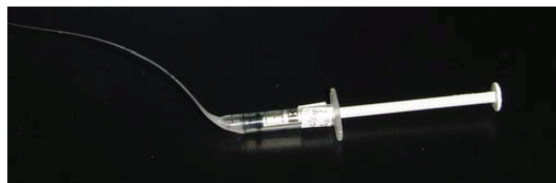
Figure 5.7. Devices for fabrication and filling of glass recording electrodes.
